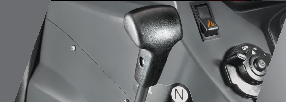
Sync-Shuttle for easy Forward Reverse operation in Puddling
