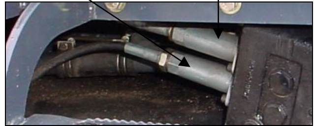
Install Dump and Rollback (Tilt) Cable to Lower Spool of Valve
