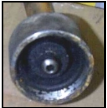
Fig. 69 OVERHEATED & CARBONED FROM LEAKING C-E RING
