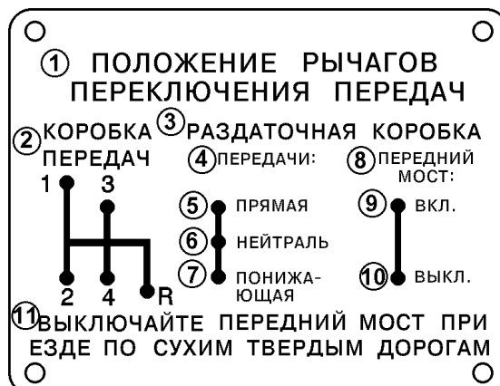
Fig.8. Instruction Plate. Positions of Transmission, Transfer Case and Front Axle Shift Levers:
