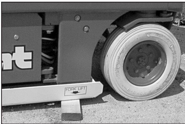
Figure 2—Pothole protector interlock test
