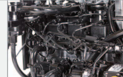
High pressure common rail fuel system to reduce the amount of PM generated during combustion.
