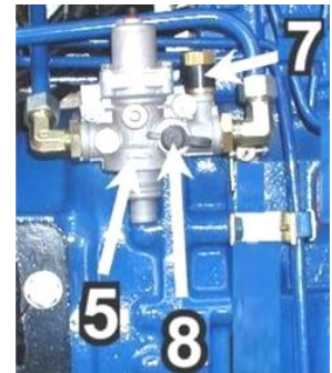
Fig. 5.13.4. Air Pressure regulating valve. 5-Air regulating valve. 7- Safety valve. 8-Tyre inflating valve.
