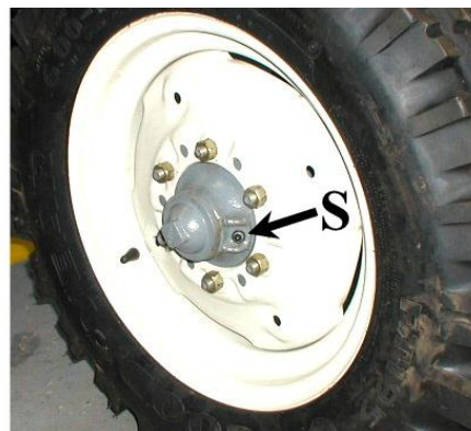
Fig. 5.7.7. Front wheel bearing grease point (non-drive axle).
