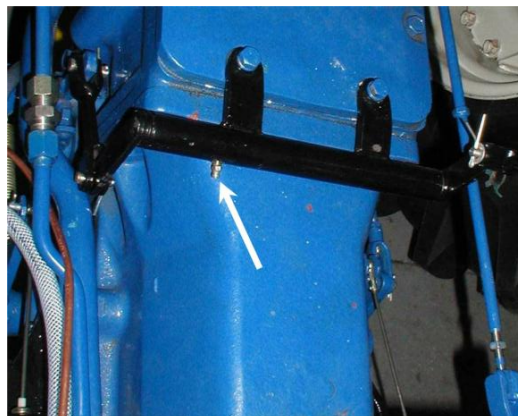
Fig. 5.8.2. Grease point of shuttle control shaft.
