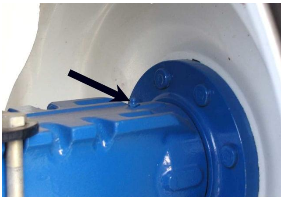
Fig. 5.7.6. Rear wheel bearing grease point.
