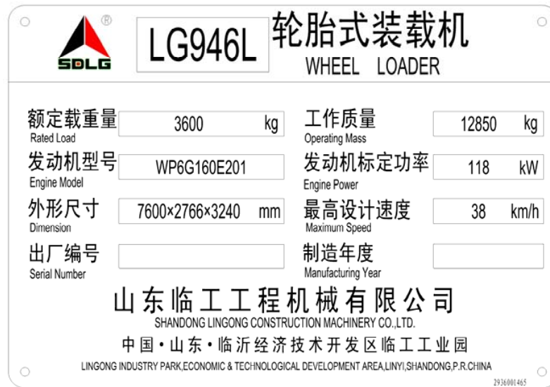
Figure 2-4 Nameplate of LG946L loader mounted with Weichai engine and enlarged lift arm
