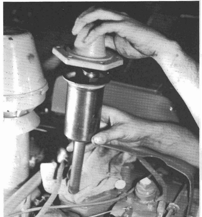
Fig. 47 Hydraulic oil filter removal
