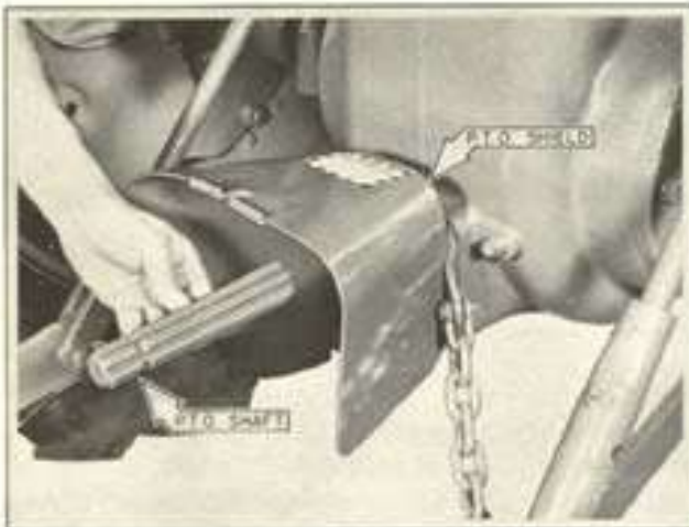
Figure 10-3 Installing Power Take-Off Shaft
