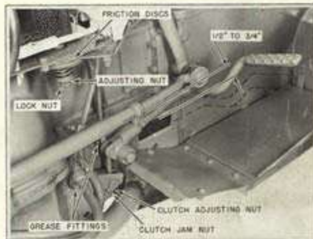
Figure 6-1 Clutch Pedal Adjustment
