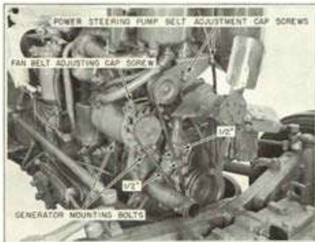
Figure 5-5 Fan Belt Adjustment
