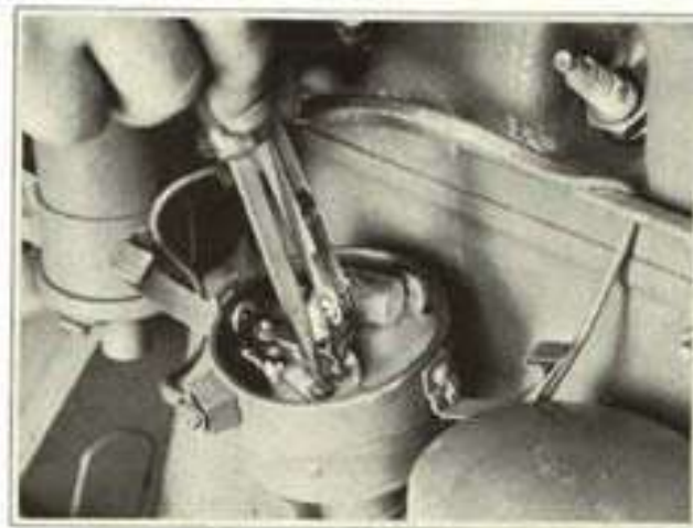
Figure 4-9 Adjusting Distributor Points
