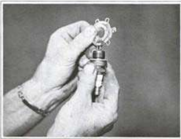
Figure 4-6 Checking Spark Plug Gap
