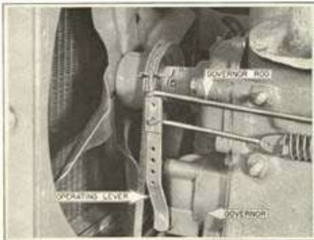
Figure 3-6 Governor Linkage Adjustment
