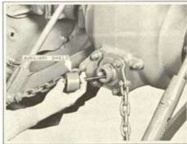
Figure 10-4 Installing Power Take-Off Auxiliary Shield
