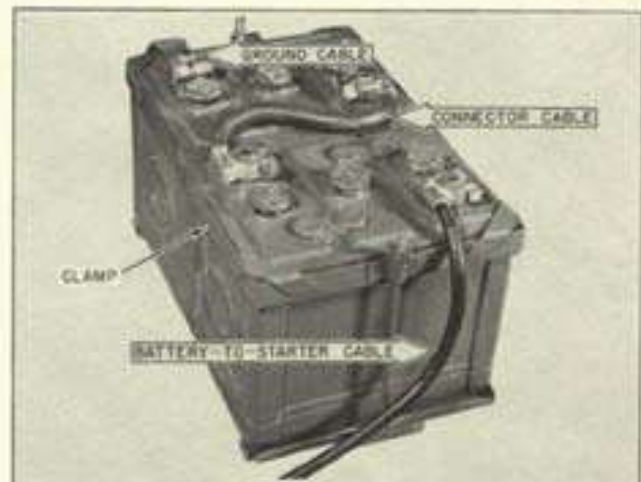
Figure 4-5 Batteries Connected For Diesel Installation
