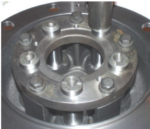
Picture 13. Installation of the planet gear shafts.
