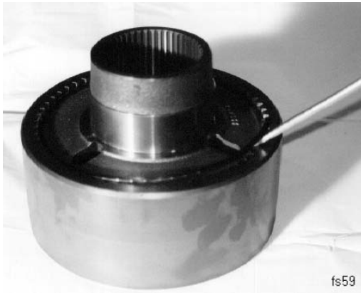
Picture 9. Retaining ring removal.
