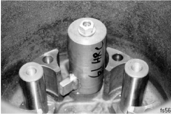
Picture 6. Planet gear shafts removing with a special tool.
