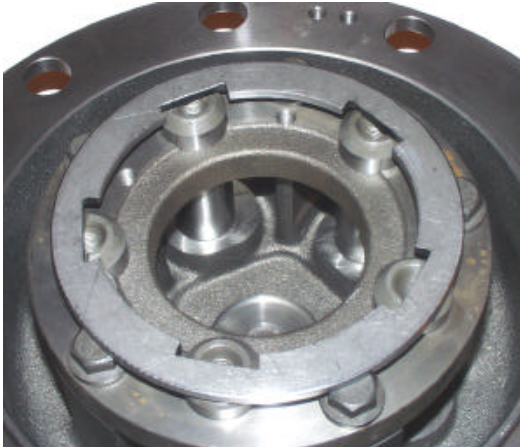
Picture 12. Positioning of the planet gear shafts
