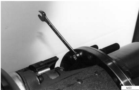
Picture 2. Unscrewing hub housing retaining screws.
