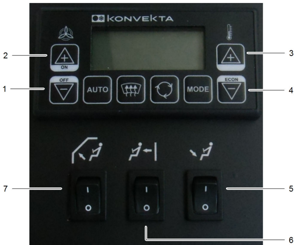
Fig. 114: Control unit for heating and air conditioning unit
