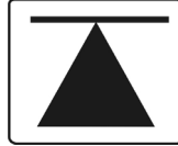
Figure 5.6.1 – Sign of a place for leveling jack installation
