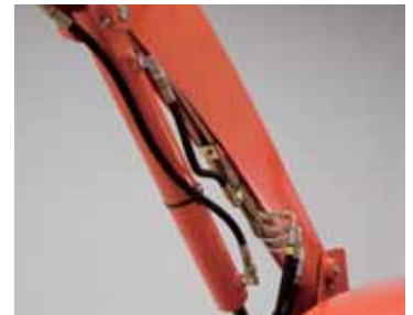
Protected Cylinder Tubes
