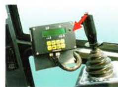
3 dimensional electric angle indicator with drilling depth and inclination
