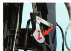
Guide swing angle indicator by pendulum
