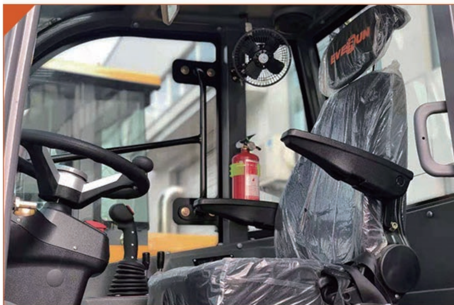
• ROPS & FOPS cabin with maintenance port
