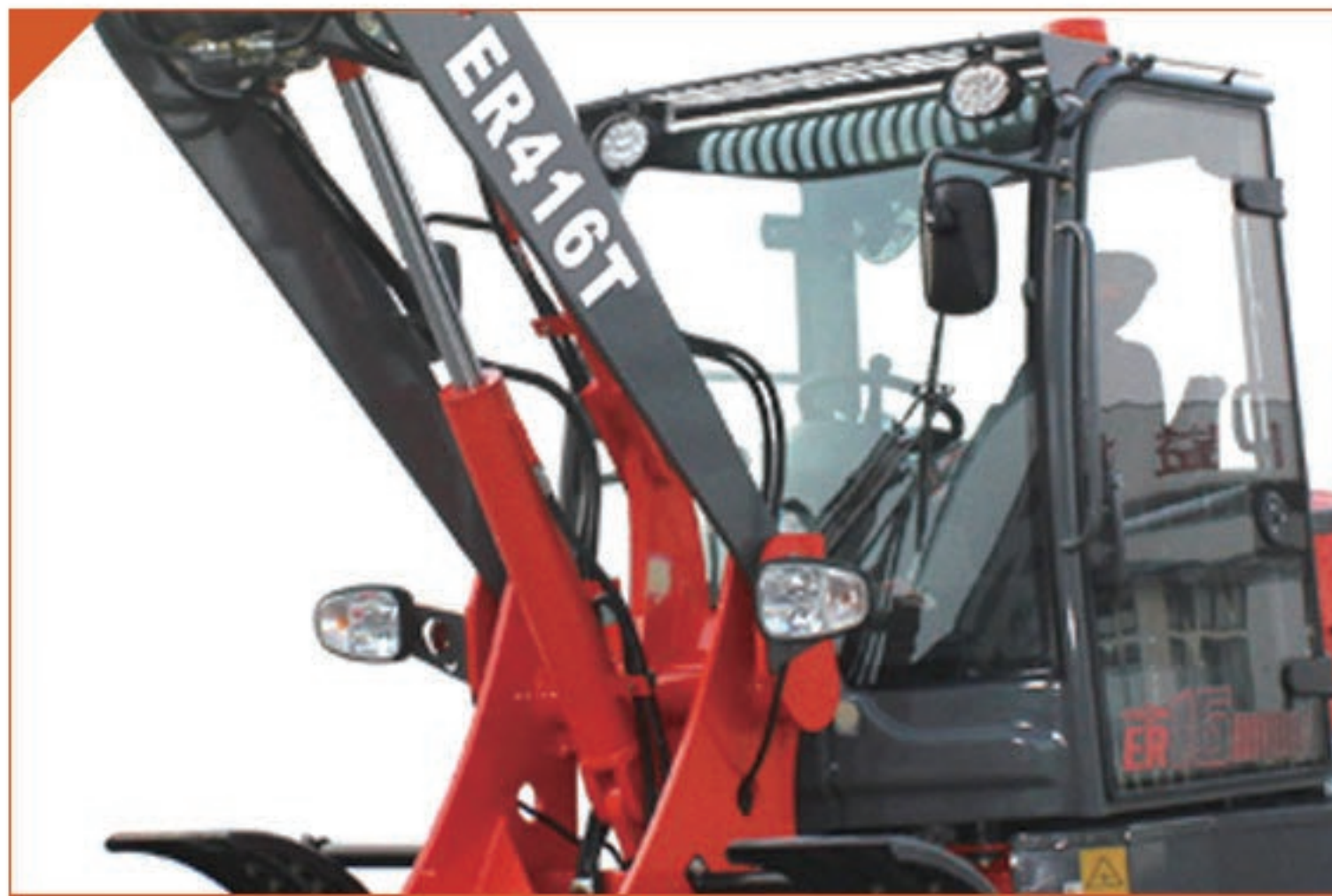
• One bigger and stronger lift cylinder
