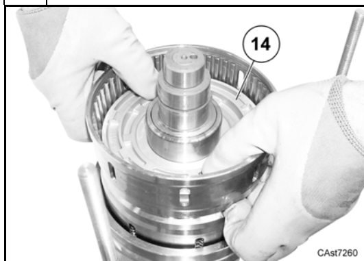
Assemble piston (14) in its seat.
