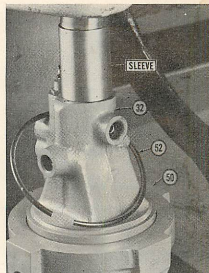
Fig. O36 — To reinstall cover retaining snap ring (52), place unit in arbor press and push housing (32) into cover (50) with sleeve as shown.
