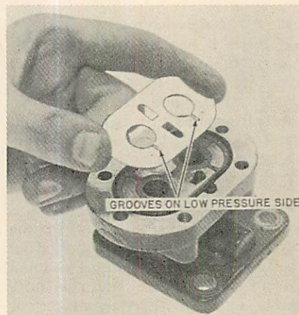
Fig. O28 — Install diaphragm with bronze side up and grooves towards low pressure side of pump as shown.
