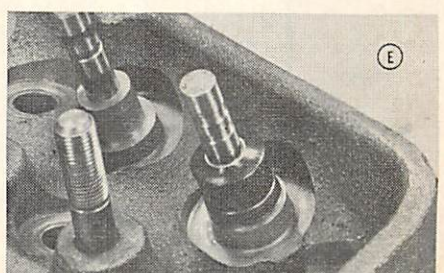
Fig. O58 — Views A through E illustrate method of installing Perfect Circle valve stem seals on models so equipped. Photos courtesy of Perfect Circle Corporation.
