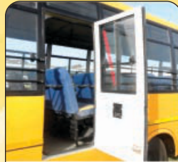
Emergency Exit Door
