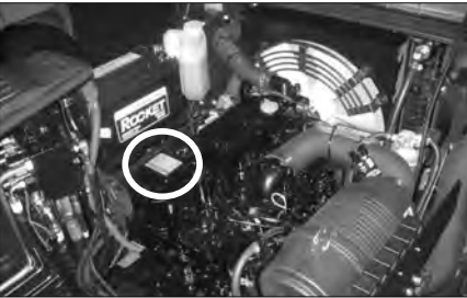
3.3 liter Diesel Engine (4TNV98) Serial Number
