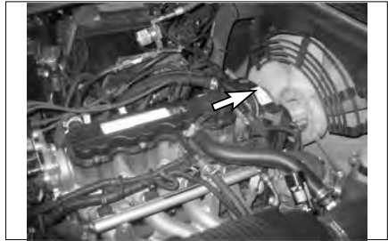
2.4 liter Spark-Ignition Engine Serial Number (G424F(E))
