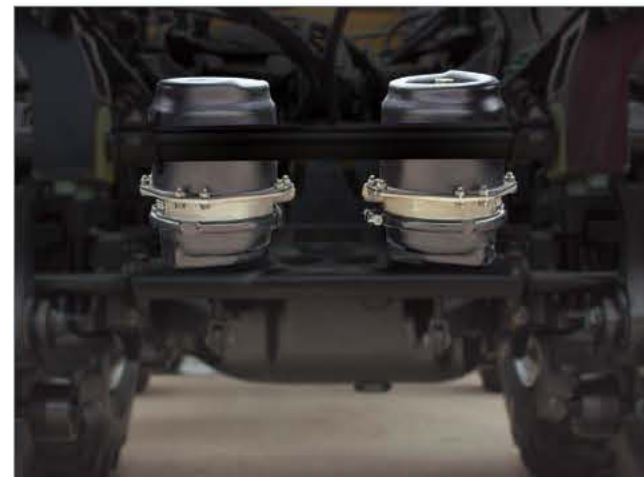
Elevated brake chambers
