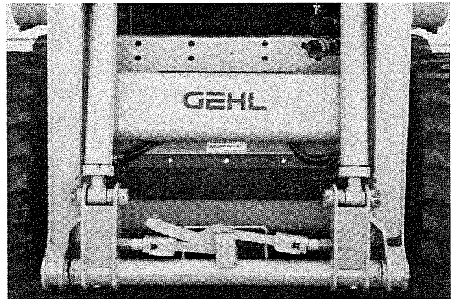
Fig. 9: Quick-Tach Lever in "Release" Position all the way to the Right (Attachment Removed for Clarity)
