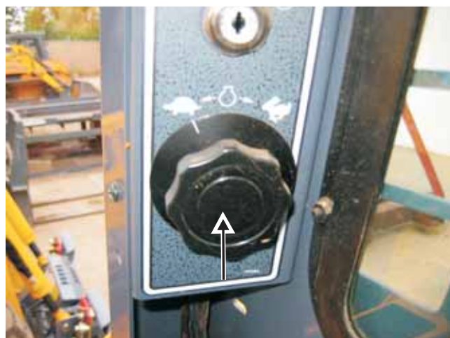
Fig. 9-30 Location of the electronic rotary throttle on the right instrument panel
