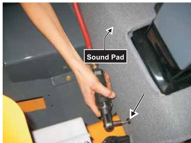
Fig. 4-18 Location of one of three screws securing the sound pad to the control cover
