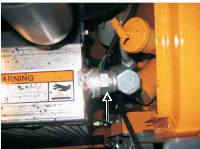
Fig. 10-26 Location of one hydraulic oil hose at top right of the cooler
