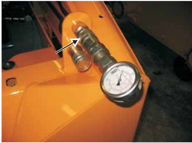
Fig. 8-9 System pressure test location on the left lift arm for standard flow hydraulic couplers
