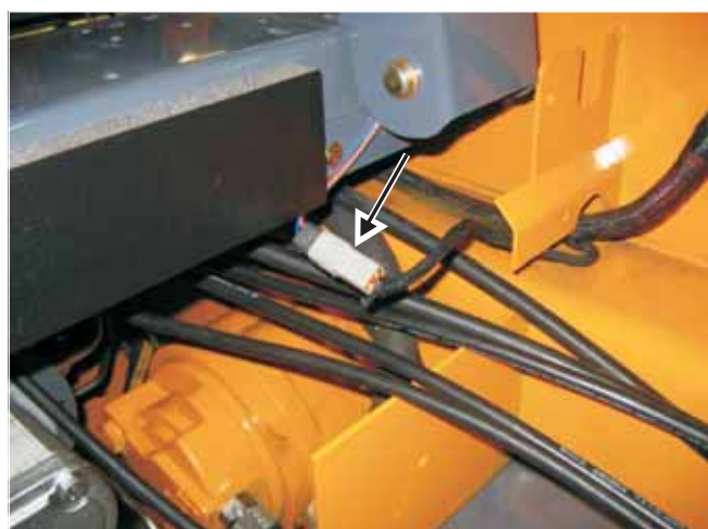
Fig. 4-26 Left control handle electrical connector underneath the crossmember, right side same
