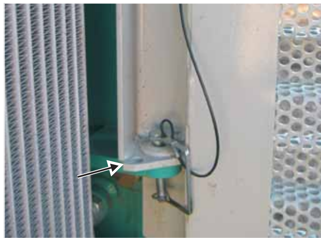
Fig. 4-29 Rear grille lock pin shown in its storage position. The hole visible in the welded tab in front of the pin keeps the rear grille from closing.
