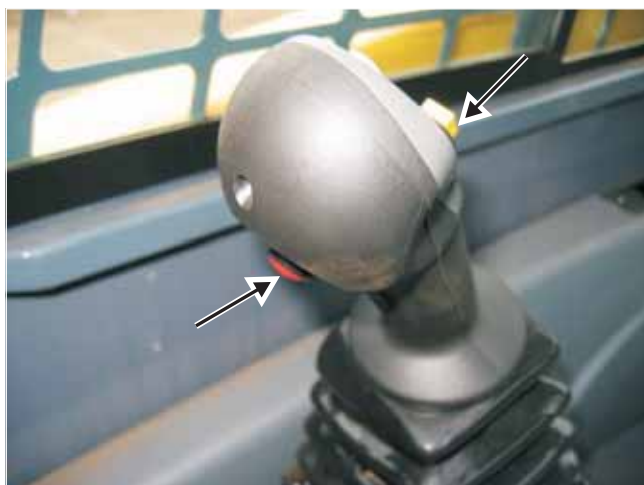
Fig. 9-23 Location of the standard-flow auxiliary hydraulics slide and trigger switch on the right control handle
