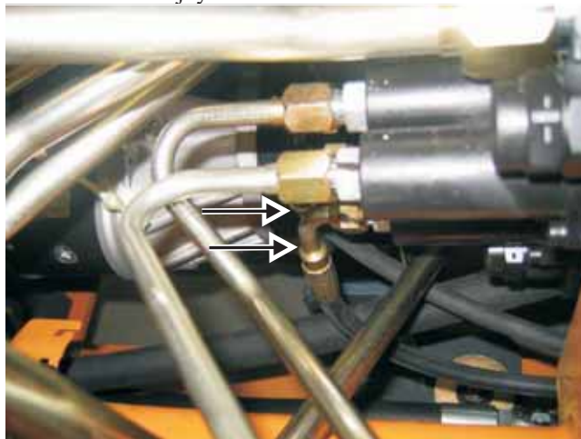
Fig. 6-11 Location of two hoses at the rear of the control valve that help control lift and tilt functions on dual joystick and t-bar/joystick control units
