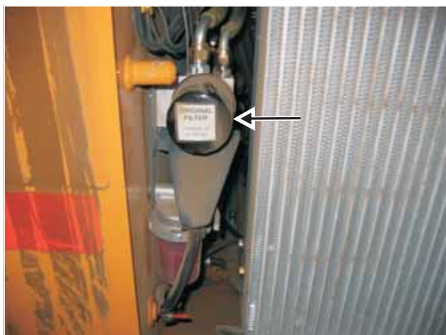
Fig. 3-6 Engine oil filter access location behind the rear grille and left of the cooler/radiator
