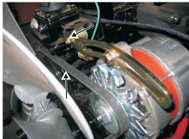
Fig. 10-21 Location to push on the belt. Also, the bolt on alternator bracket attached to the engine
