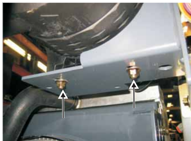
Fig. 10-11 Unbolt two capscrews and locknuts securing air cleaner clamp to the chassis
