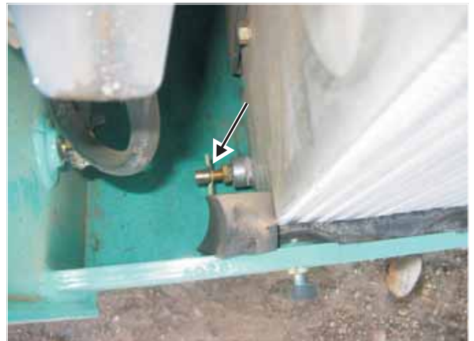
Fig. 3-11 Location of the anti-freeze drain cock located at the bottom left on the radiator/cooler
