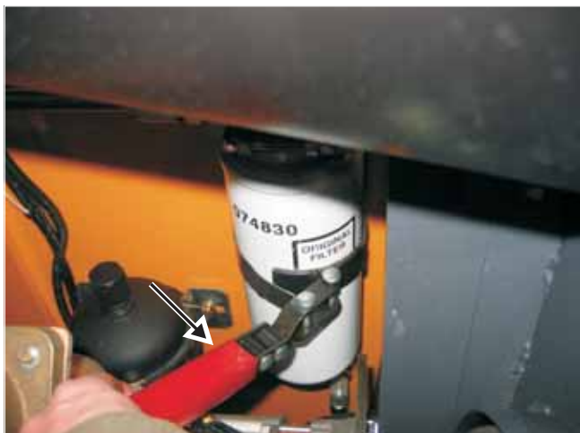
Fig. 8-16 Use a filter wrench on the element and turn the element counterclockwise to remove, clockwise to install
