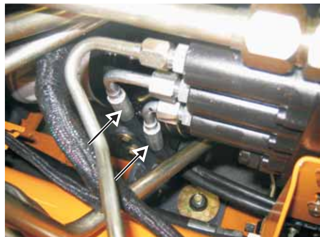
Fig. 4-23 Location of two hose lines at rear of the control valve joined to the right dual joystick control handle
