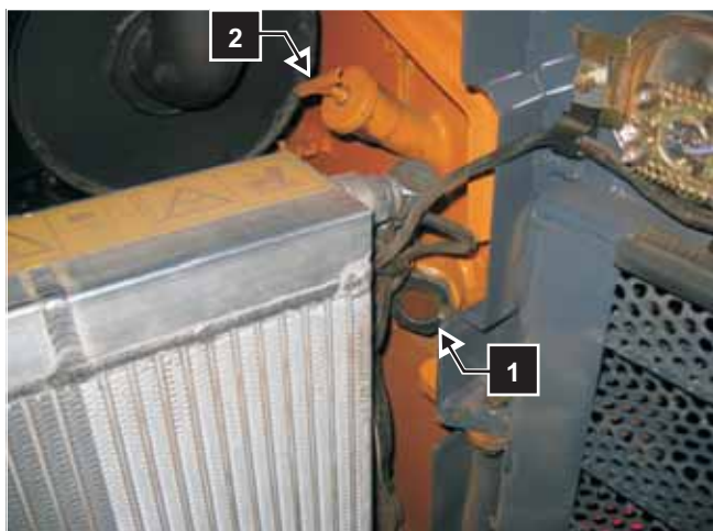
Fig. 3-1 Hydraulic oil level indicator (1) and hydraulic oil fill (2)
