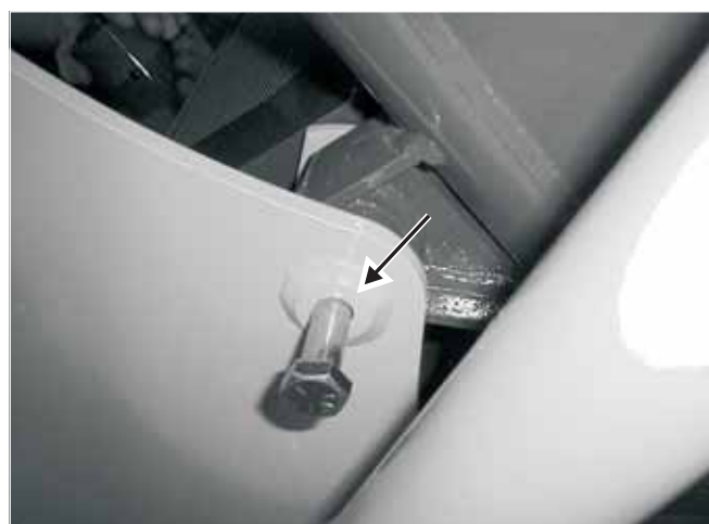
Fig. 4-5 View of ROPS bolt turned out just enough to release the engine access cover, but not enough to release the ROPS
