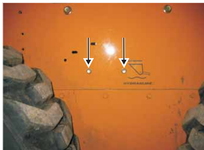
Fig. 8-29 Location of two locking capscrews securing the manifold valve to the right side of the chassis wall
