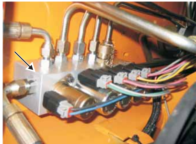
Fig. 8-27 View of 5-bank high-flow manifold valve on inside right of the chassis. Note the many electrical connectors attached to it
