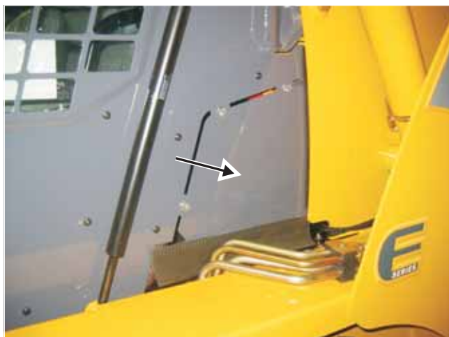
Fig. 3-5 Battery access location behind the left engine side cover
