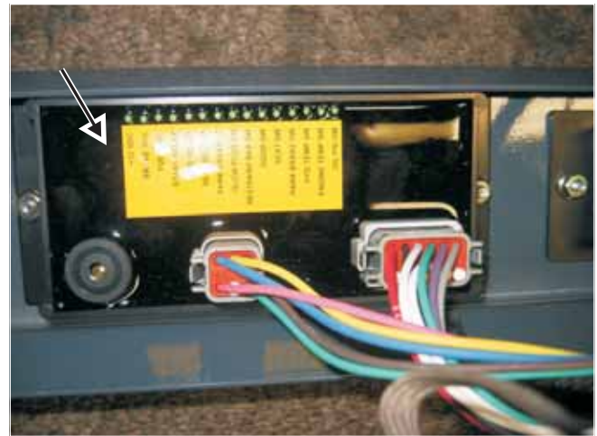
Fig. 9-15 Location of the interlock control module inside the left instrument control panel
