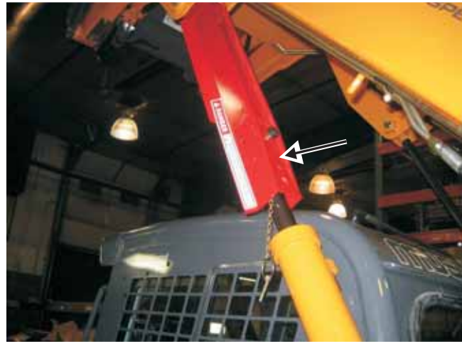
Fig. 2-4 The lift arm support device dropped over and around the cylinder rod
