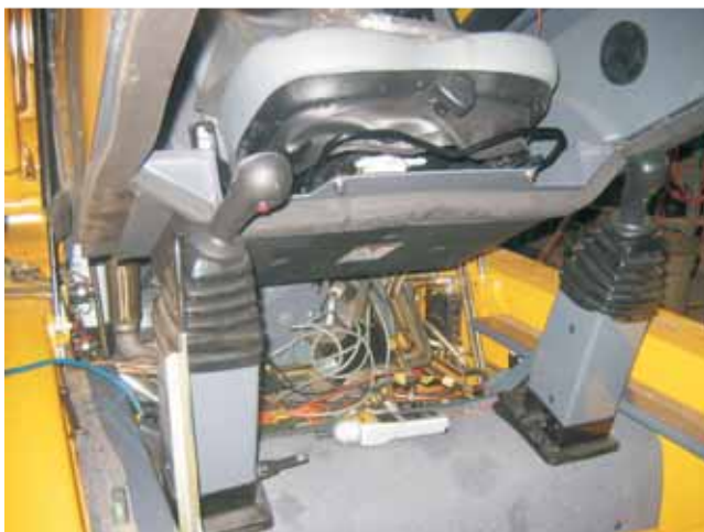
Fig. 2-9 Be sure control handles clear the ROPS
