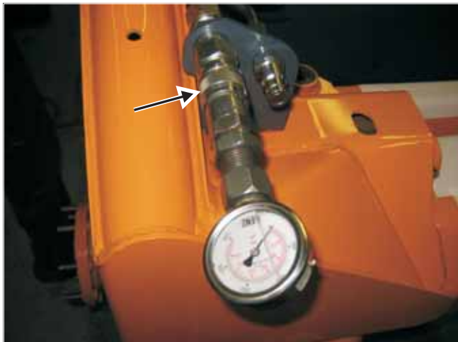
Fig. 8-10 System pressure test location on the right lift arm for high-flow hydraulic couplers
