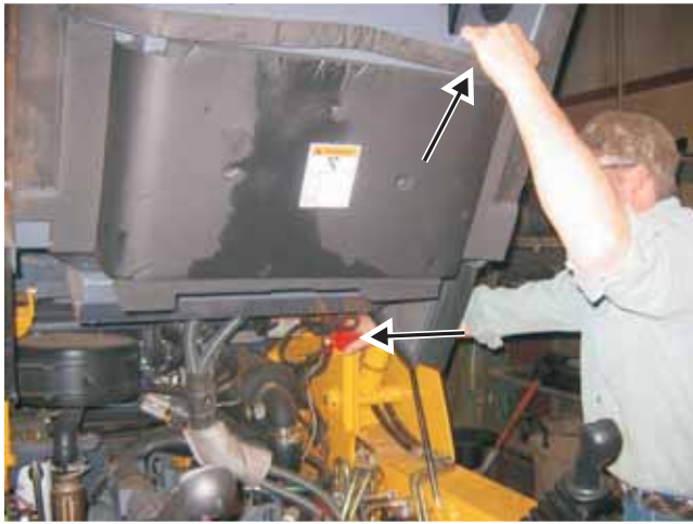
Fig. 2-7 Push up on ROPS to release locking mechanism
