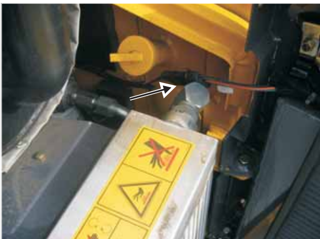
Fig. 4-28 Location of the rear grille lights connector
