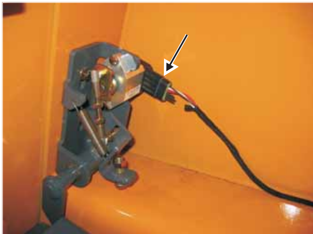
Fig. 6-16 Unplug this electrical wire connector from the throttle assembly
