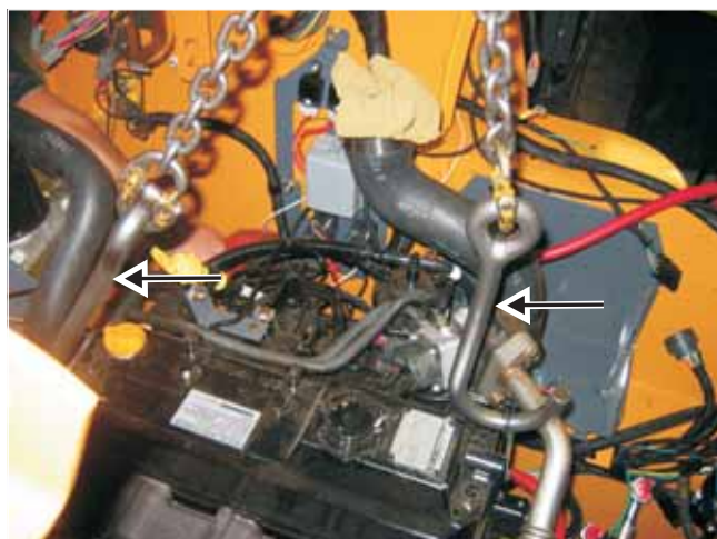
Fig. 10-43 Lift hooks on lift eyes on the engine are ready to pull the engine out of the skid-steer loader
