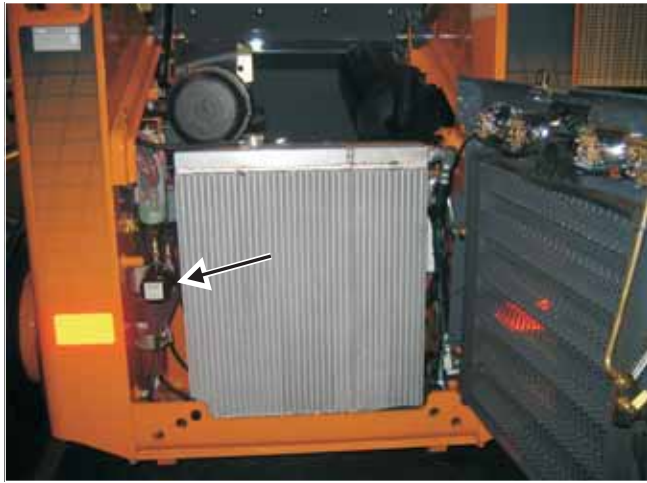
Fig. 10-6 Remote engine oil filter access point on the left side of the radiator cooler
