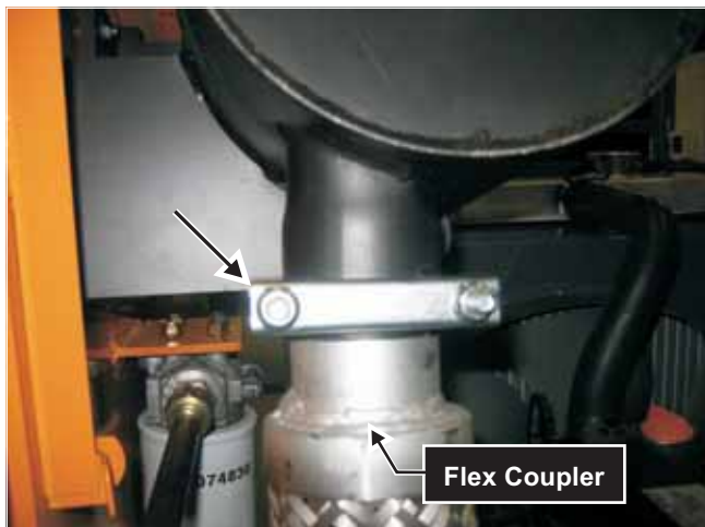
Fig. 10-18 Location of muffler clamp securing muffler to flex coupler
