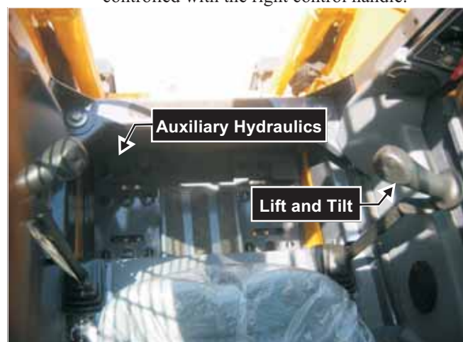
Fig. 2-12 On Dual T-Bar models, lift and tilt functions are controlled with the right control handle. The auxiliary hydraulics are controlled with the left foot on the auxiliary pedal assembly.
