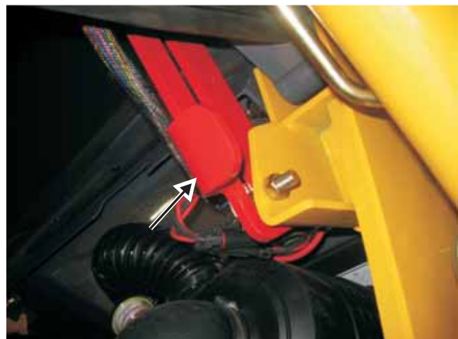
Fig. 2-6 Location of the self-actuating lock mechanism
