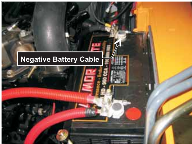
Fig. 10-12 Disconnect the negative battery cable first, then, disconnect the positive battery cable
