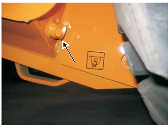
Fig. 3-2 Hydraulic oil drain plug located behind the right rear tire
