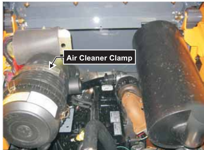
Fig. 10-9 View of air cleaner assembly from rear of skid-steer loader
