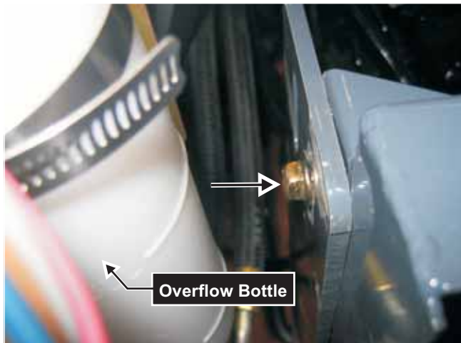
Fig. 10-30 Location of one of five flange screws securing the shroud assembly to the cooler mount plates, other side same
