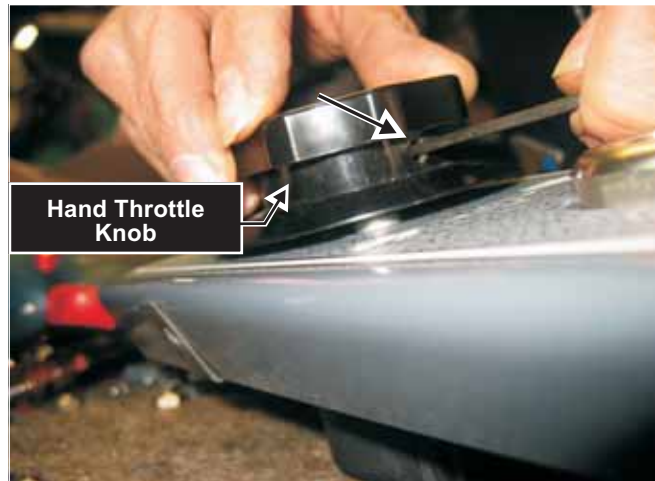
Fig. 6-12 An Allen wrench is used to loosen the set screw on the hand throttle control knob
