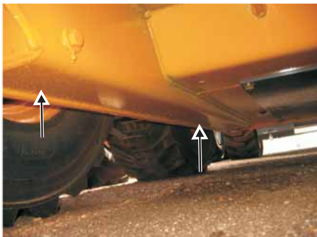
Fig. 2-15 Location underneath the right rear skid loader to position stands or blocks. View is from the rear of the loader.
