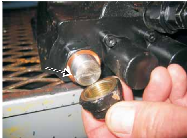
Fig. 8-13 View of the adjuster screw beneath the cap on the relief valve
