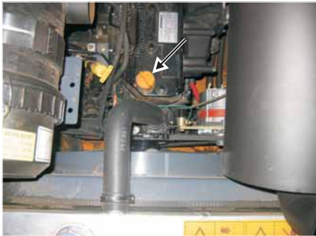
Fig. 3-8 Location of engine oil fill
