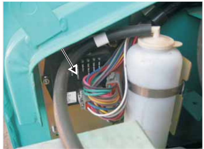
Fig. 9-18 Location of the two-speed, ride control and float module inside the engine compartment
