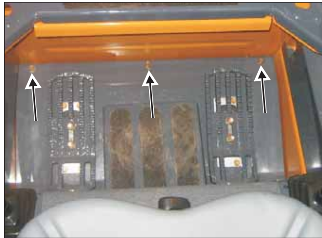
Fig. 6-7 Location of three of five capscrews securing floor plate to the chassis
