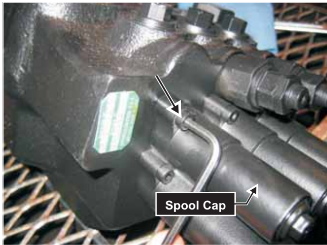
Fig. 8-30 View of a hex socket capscrew, 1 of 2, used to securing the spool cap to the control valve
