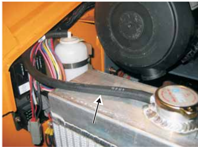
Fig. 10-27 View of the radiator cooler overflow line connected to the overflow bottle
