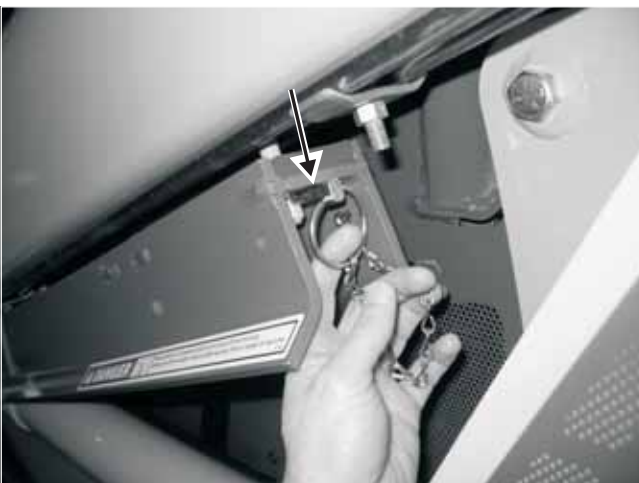
Fig. 2-3 Pull ring out of welded post
