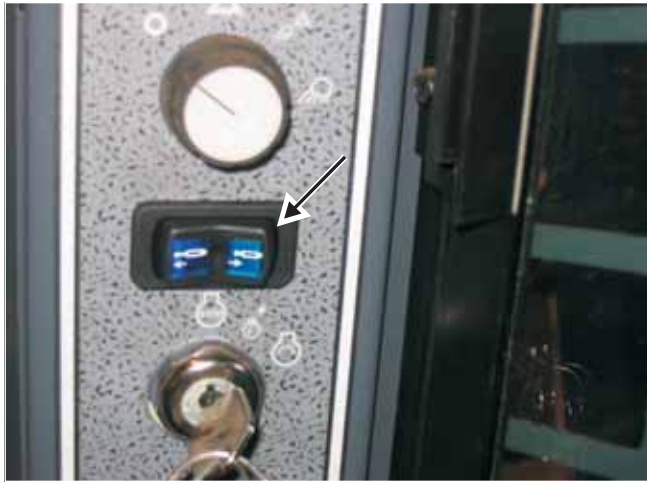
Fig. 9-28 Location of the high-flow auxiliary hydraulics control rocker switch in the right instrument panel
