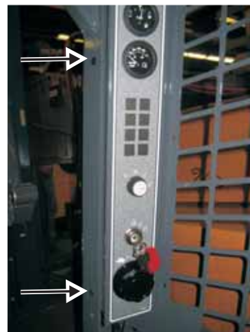
Fig. 6-14 Location of two of three machine screws securing the right instrument panel in the ROPS stanchion
