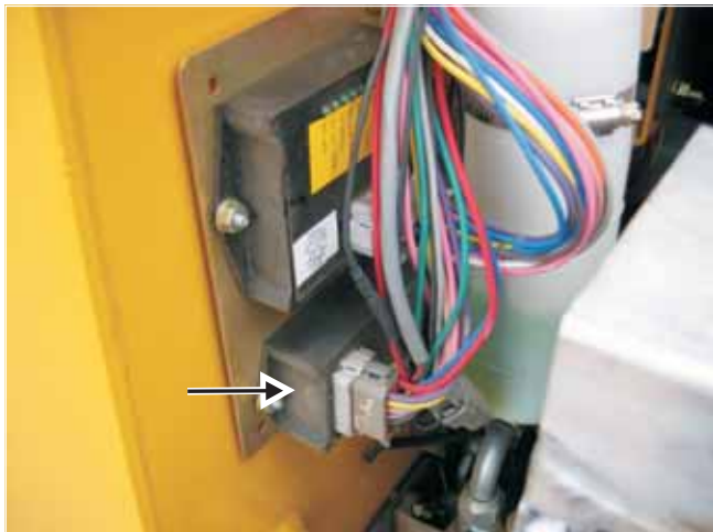
Fig. 9-29 Location of the high-flow auxiliary hydraulics high-flow module
