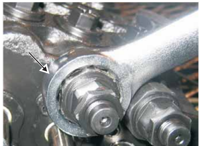
Fig. 8-33 A wrench can be used to remove a port relief valve from the control valve body
