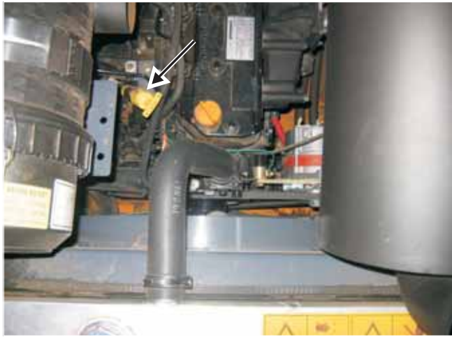
Fig. 3-7 Location of engine oil dipstick
