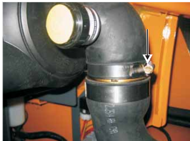
Fig. 10-10 Location of hose clamp to loosen at the front of the air cleaner
