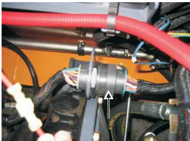
Fig. 10-39 Unplug the engine harness at this location
