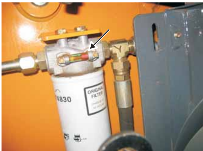
Fig. 3-9 Location of the hydraulic filter indicator underneath the muffler
