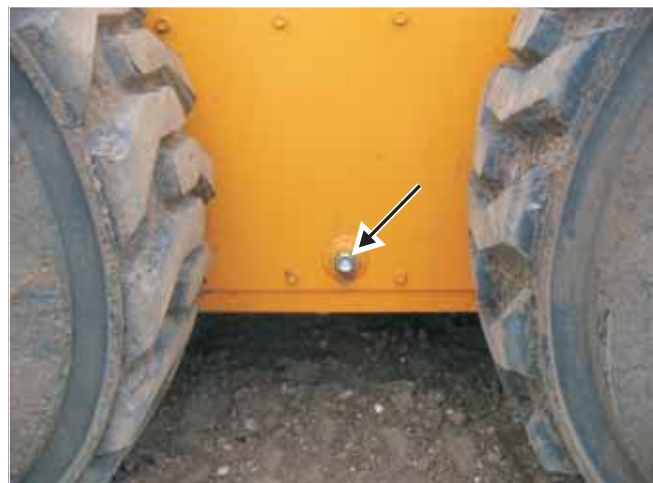
Fig. 3-12 Location of the left chaincase oil fill plug. Right side same
