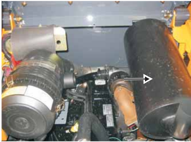
Fig. 10-17 Location of muffler in the engine compartment
