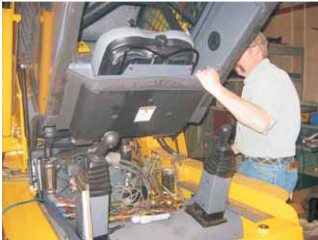
Fig. 2-8 Lower the ROPS until it contacts the chassis
