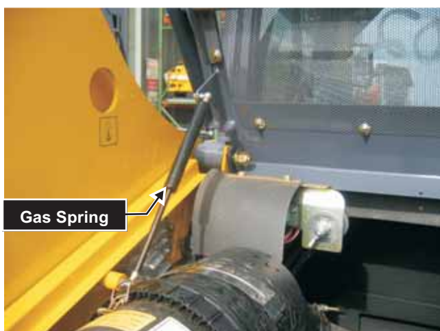
Fig. 4-2 View of the gas spring that supports the engine access cover
