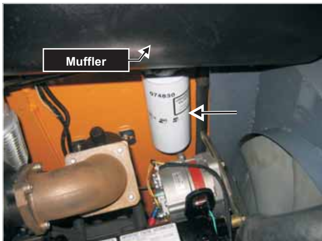
Fig. 8-15 Location of the hydraulic oil filter on the right riser, below the muffler
