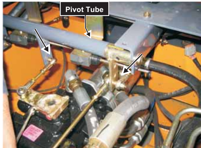
Fig. 4-21 Disconnect wheel drive control rods at pivot tube on hand/foot, t-bar and t-bar/joystick units
