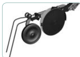
Double disc unit and depth gauge wheel.
