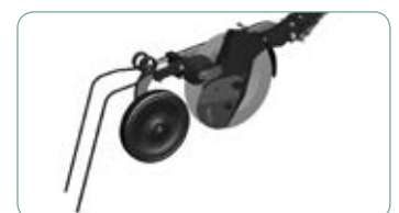
Single disc unit and depth gauge wheel.
