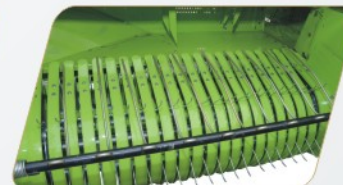
Using Steel Pick-up Guard
