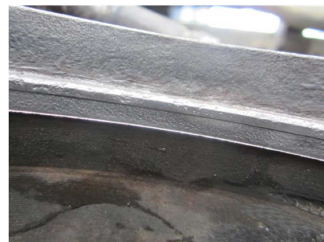
Unacceptable damaged liner bore
