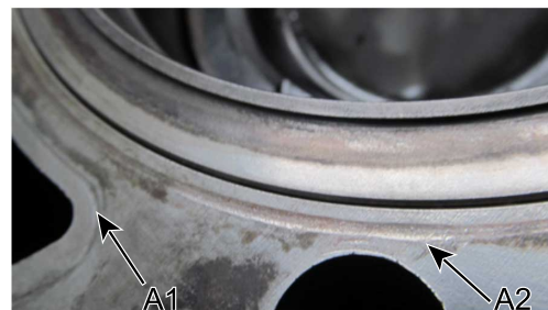
Acceptable damaged top deck
