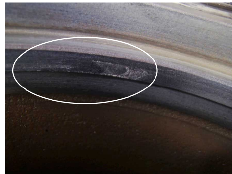
Acceptable damaged liner bore
