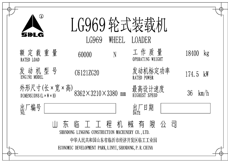
Figure 2-4 Nameplate of LG969 wheel loader mounted with standard lift arms
