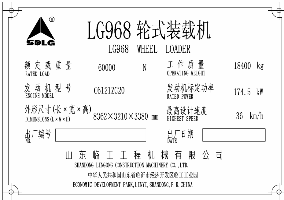
Figure 2-3 Nameplate of LG968 wheel loader mounted with standard lift arms
