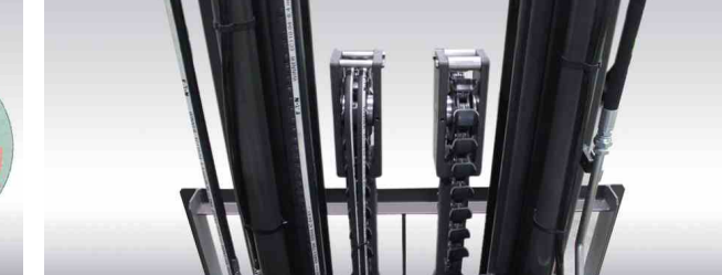
Mast triple full free equipped with double front cylinder, increasing greatly the driver operating field of vision.
