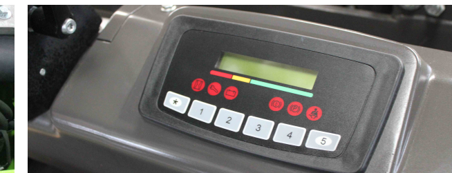
With multi-function LCD display users can easily monitor the performance and working status of the vehicle through the information displayed on the display.
