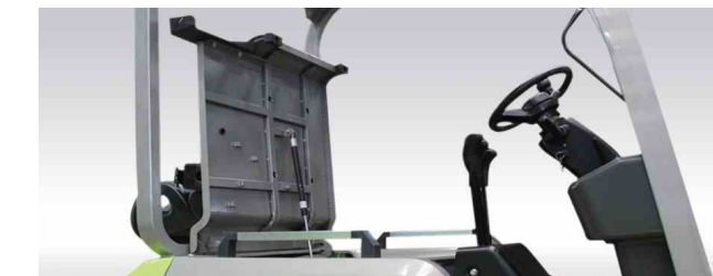
The battery cover adopts hydraulic tappet support, it can be fully opened, easy to maintain the battery.
