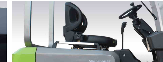
Advanced suspension seat with suspension damping function, which can ease the driver fatigue, and improve work efficiency.
