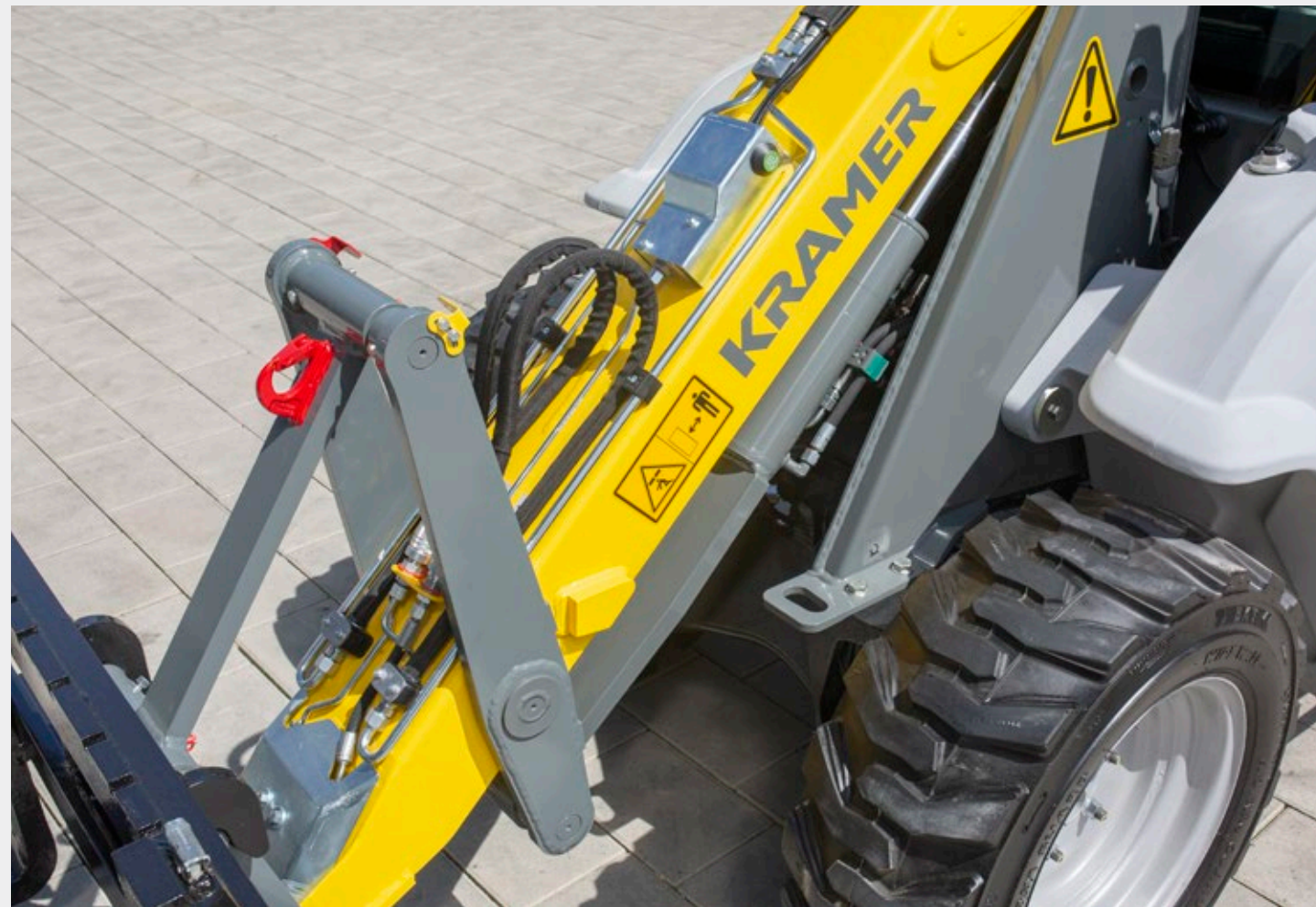
Sturdy loader unit with Z-kinematics, visual position display and optional load hook.
