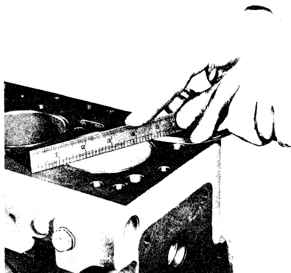
G2 Method of checking Liner protrusion.
