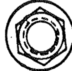
(1) Locknut 5/16"-18 For Adapter STD541431
