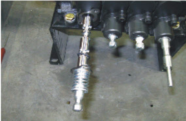
Figure 3-6 Hydraulic Valve Disassembly
