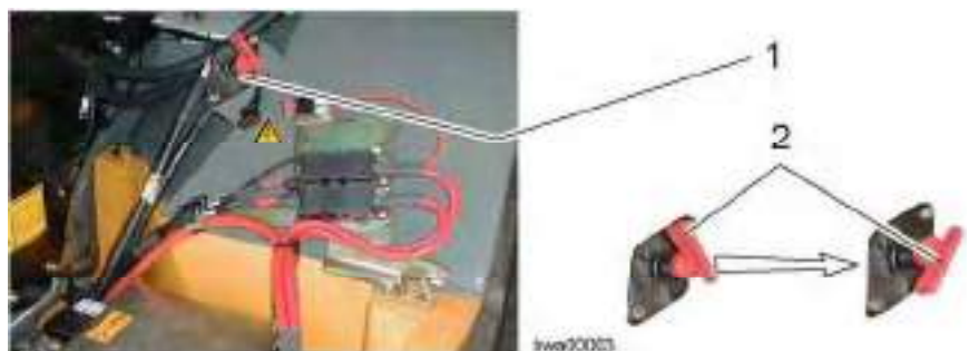
Turning off the battery main switch
