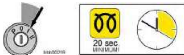
Ignition key contact and preglow positions
