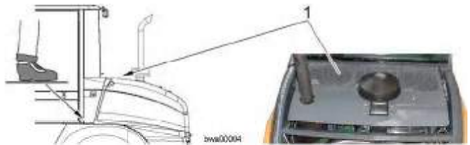
Cooling system grille
