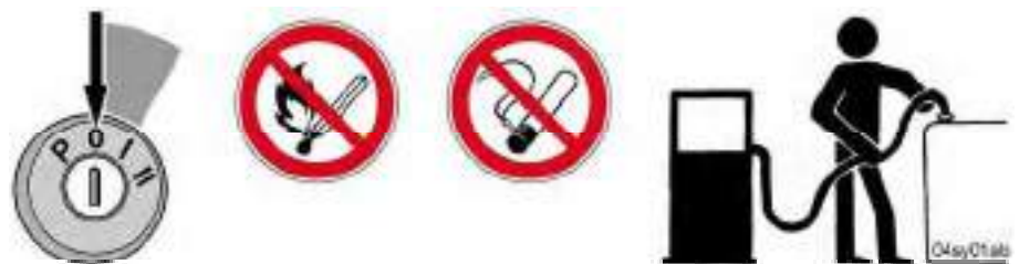
Safety while refuelling
