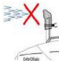
Blocking off the exhaust pipe opening
