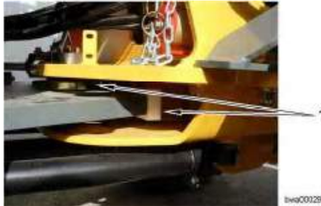
Lubricating the articulation bearing and rear oscillating bearing
