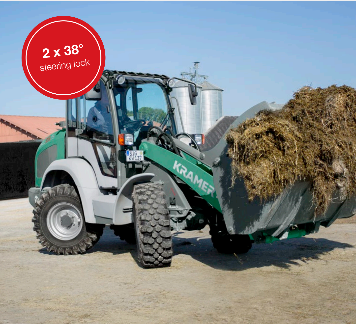
All-wheel steering: particularly manoeuvrable in tight spaces
