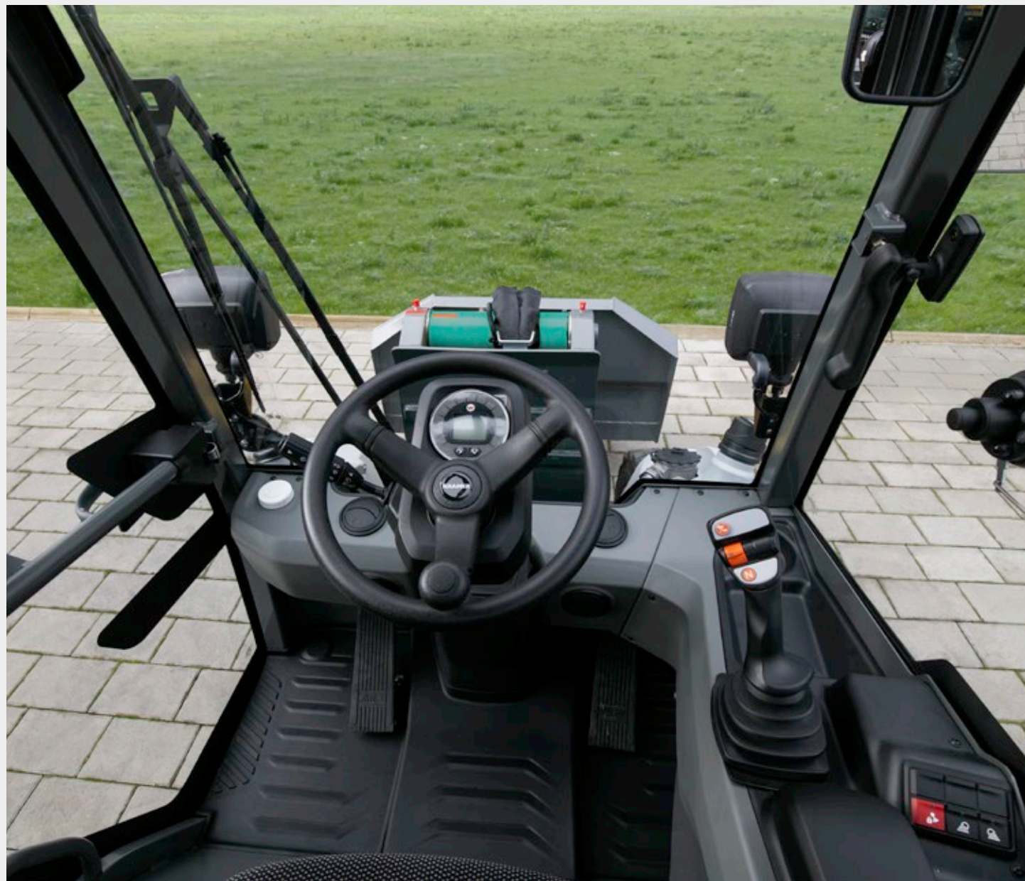
Comfortable joystick: Possible to switch between hare and tortoise on the joystick itself.
