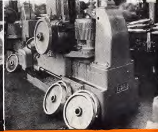
This giant machine cuts several tractor bull gears in a single operation. It is typical of the equipment used throughout the entire Oliver "Cletrac" factory.
