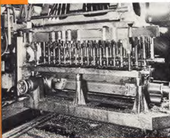
This multiple drilling machine drills 43 holes in one operation—it not only cuts costs of production but it also assures perfect alignment of the holes.
