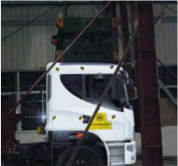
Roof pressing experiment of the cab
