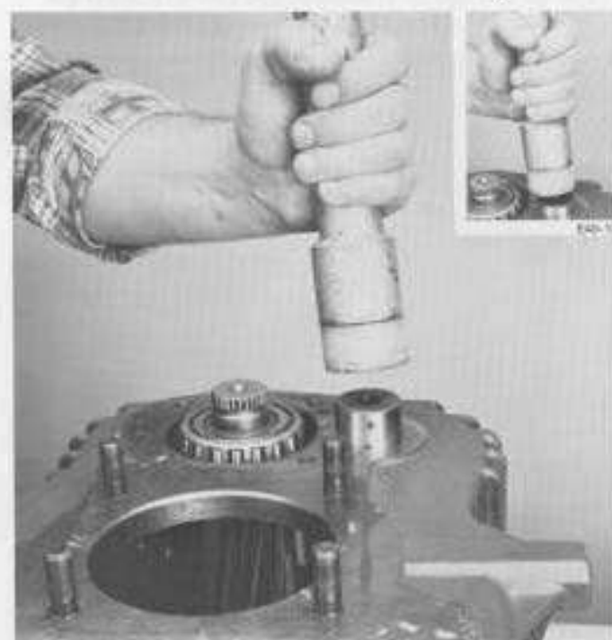
13. Insert idler shaft through case and idler gear bearings. Line up notch in shaft with notch in case, install lock ball, and drive shaft into position (inset).
