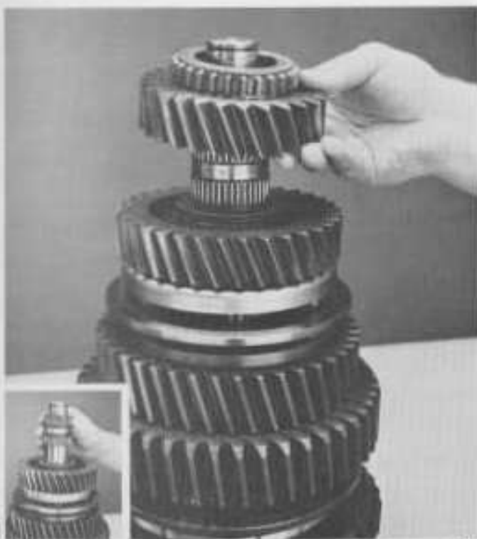
13. Lubricate and install 4th gear bearings and spacer (inset). Install 4th gear, clutching teeth facing up.
