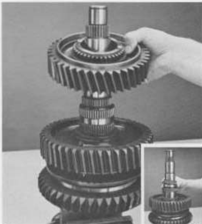
8. Lubricate and install 2nd gear bearings and spacer (inset). Install 2nd gear, clutching teeth facing up.
