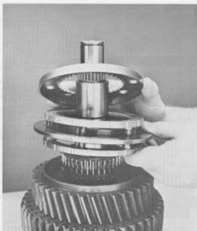
10. Remove 3rd speed synchronizer cup and 2nd-3rd speed synchronizer.
