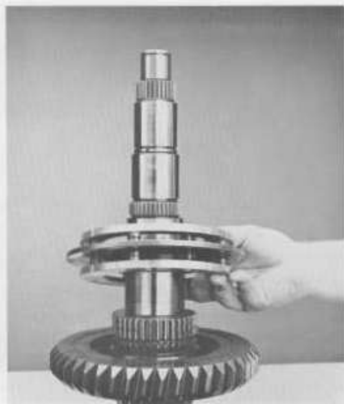
15. Remove 1st speed synchronizer.
