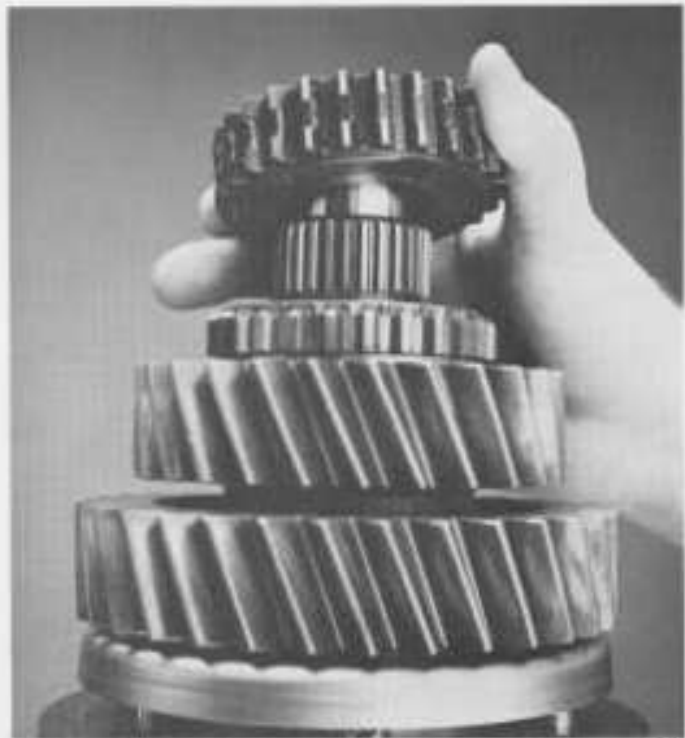
14. Install 4th-5th clutch hub with shoulder end of hub facing down.
