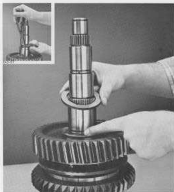
7. Install locating ball and washer. Washer can be installed either way. Install snap ring as shown (inset).
