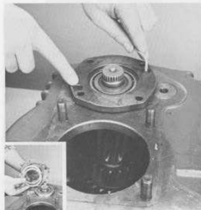
15. Temporarily install new shims into bearing retainer (inset). Install retainer. Tighten set screws to 5-10 lbs. ft. (7-14 Nm).
