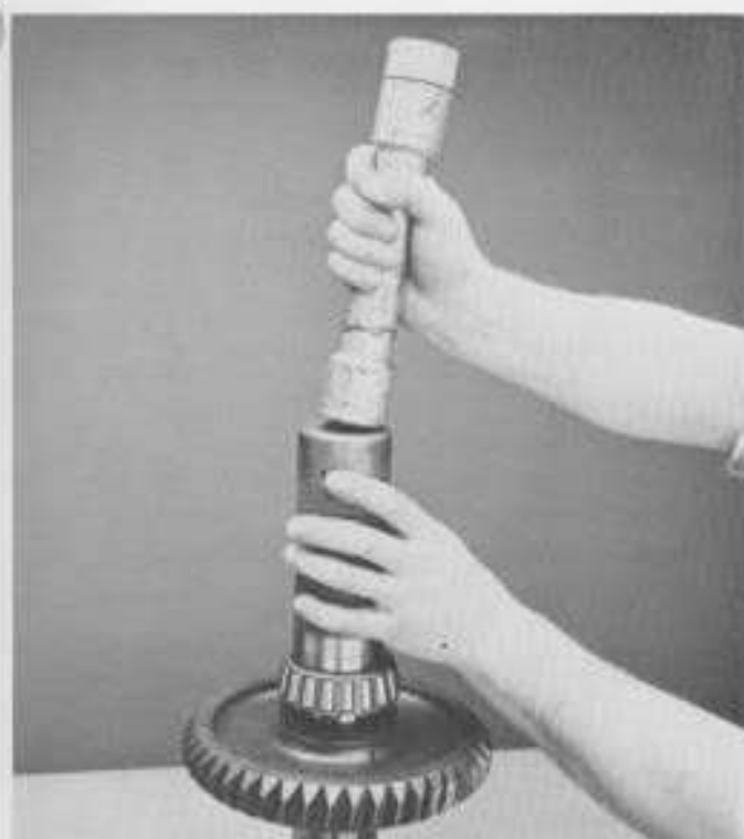
4. Using a sleeve type driver install rear mainshaft bearing as shown.
