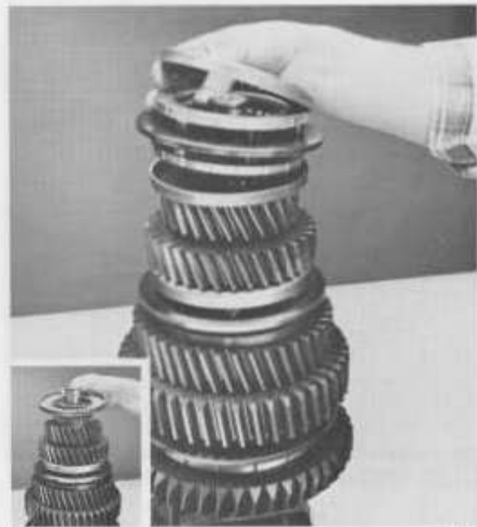
15. Install 4th speed synchronizer cup (inset). Lubricate friction surface with transmission lube and install 4th-5th speed synchronizer assembly and 5th speed synchronizer cup.
