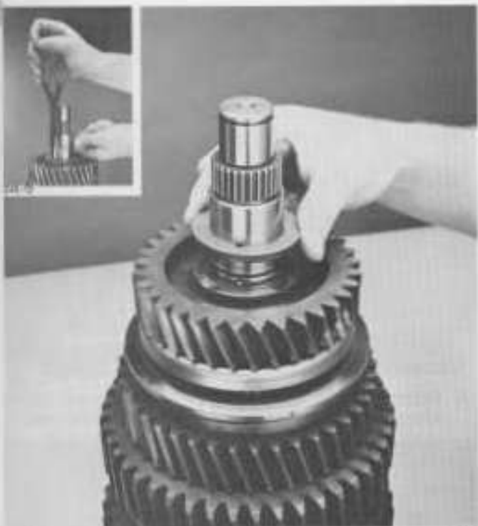
12. Install locating ball and washer. Washer can be installed either way. Install snap ring as shown (inset).
