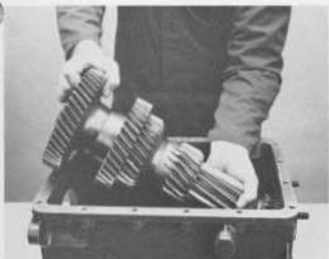
9. Carefully lower countershaft into case.
