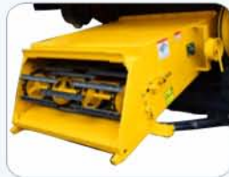
Feeder chamber length increased. Single sheet bending
