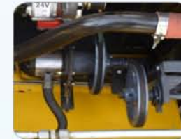
High capacity hydraulic pump used (26L).
