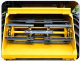
Sprocket counting increased in chamber. More feeding capacity.
