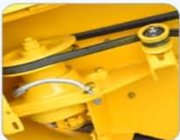
Heavy duty gear box used for oscillation of Blades.
