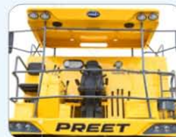
Newly design heavy duty front railing
