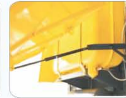
Gas spring used for opening of shields.
