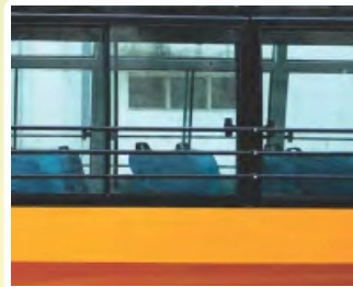
Window Guard Rails
