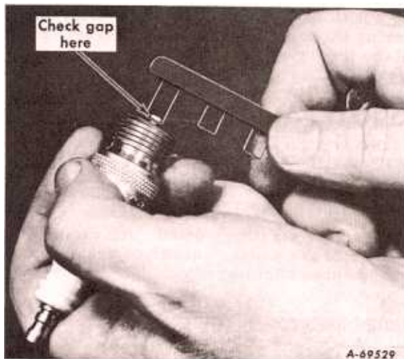
Illust. 18 Checking the spark plug gap. Set gap at .025-inch.
