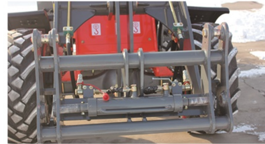
Hydraulic quick hitch to exchange attachments easily and conveniently
