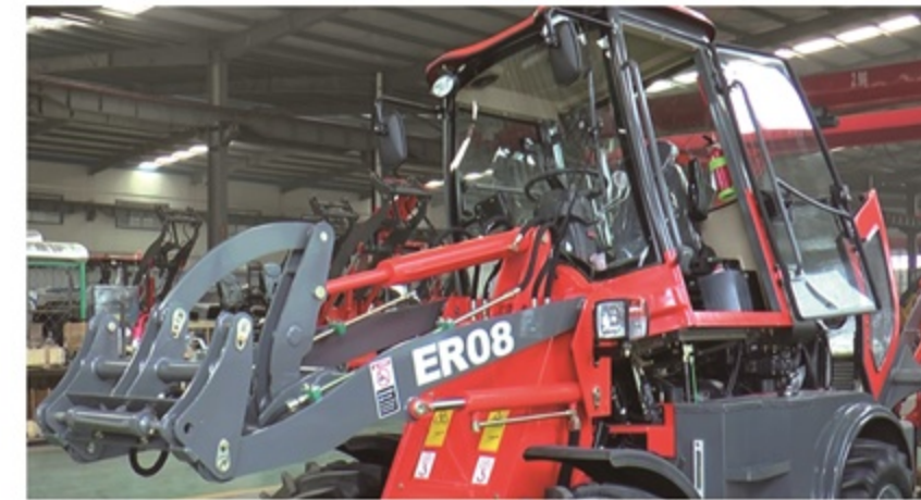
The patented Everun cab with Tilttable design meets Rops and Fops standard
