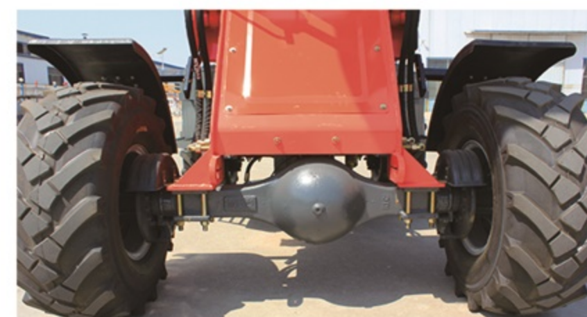
Strong axle to meet diverse terrains and traction requirements
