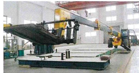
XC6-4517 has passed fatigue load and overload tests of 200,000 times
