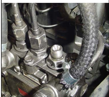
Fig. 9: Opening on fuel pump
