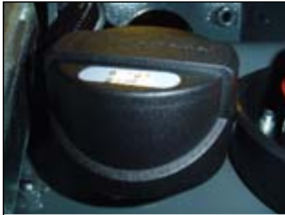
Fig. 13: Breather filter position
