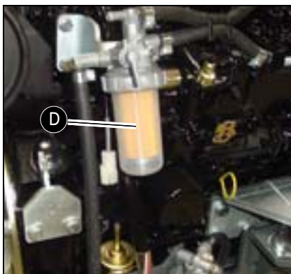
Fig. 5: Fuel filter position
