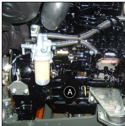
Fig. 10: Engine oil filter position
