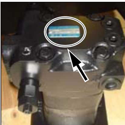
Fig. 7: Swivel unit type label
