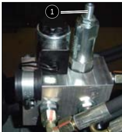
Fig. 24: Pressure reducing valve
