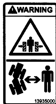
Fig. 5 WARNING! Warning, risk of crushing at frame joint if machine is steered
