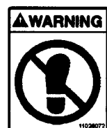
Fig. 5 WARNING! Warning, risk of crushing at frame joint if machine is steered
