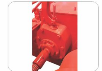
Oil-immersed brake designed for use on a drive heavy machines
