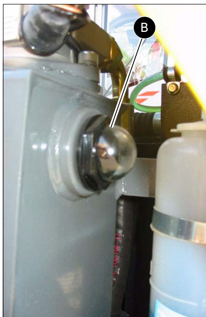
Fig. 18: Oil level indicator on the hydraulic oil tank
