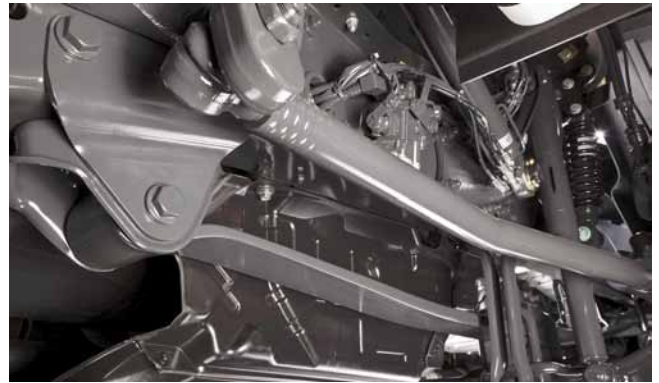
Front spring, 3.6 t, parabolic (Q1J)
