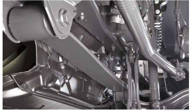
Front spring, 3.4 t, parabolic (Q1C)
