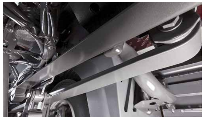
Rear spring, 5.0 t, parabolic, 1-leaf (Q2N)
