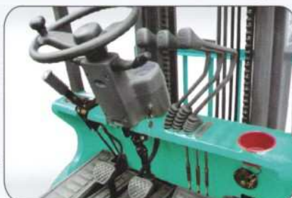
Control valve in the front
