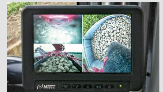
The special wide angle camera mounted on the transfer loader allows a perfect sight
