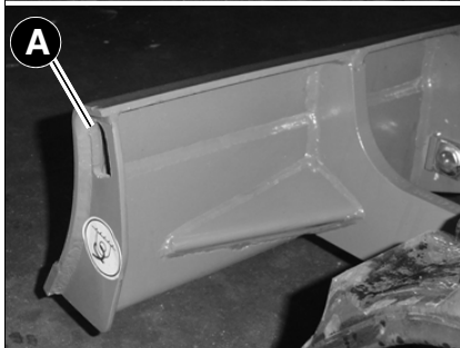
Fig. 65: Tying down the excavator
