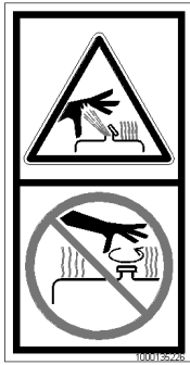
Fig. 16: Hydraulic oil tank under pressure
